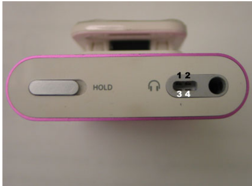
Fig 5. iPod remote controller pin configuration
